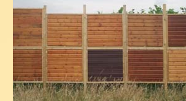
Outdoor exposure at Teknos' UK test site
